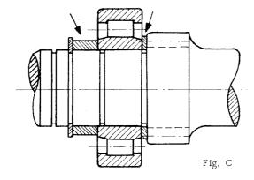
Fig. C illustrates the location of the intermediate ring and distance ring, when installed with input shaft 519.20.249 in a transmission housing 741.301.010.10.
