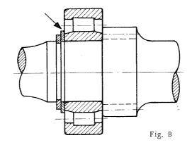
Fig. B illustrates the location of the intermediate ring when installed with input shaft 741, 302, 101, 10 in a transmission housing 644, 20, 010 or 716, 301, 010 or 741, 301, 010, 00.
