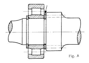
Fig. A illustrates the standard location of an intermediate ring between gear 1 for the 1st speed on the input shaft 741.302.101.10 and the roller bearing, from transmission No. 51017.
